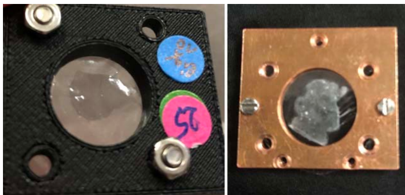
Figure 2: left: freshly prepared liquid G5P sample in sample holder. right: dried sample of G5P in sample holder
