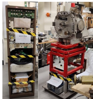
Figure 1 Electronics rack (left) and the experimental chamber (right) for CARPES setup.
