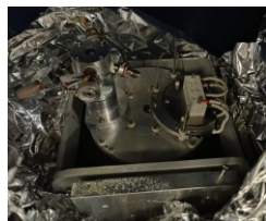
Figure 2 Hemispherical electron monochromator attached to a collision region
